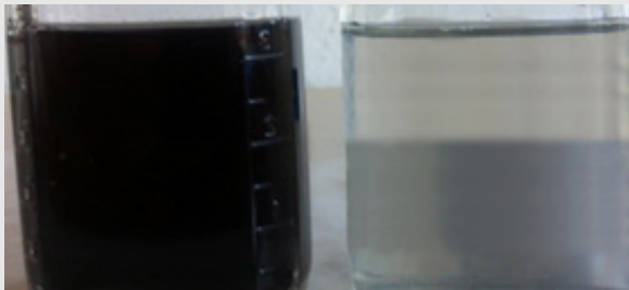
Oil bound with Iron Sulfide in water wells
